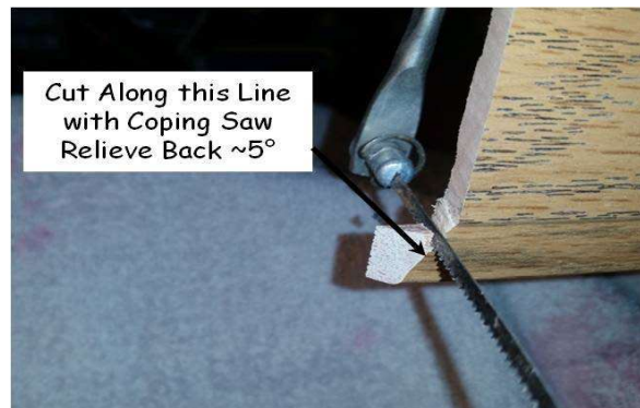
Figure 19-8. Coping Saw Cut.
