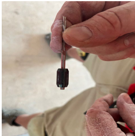
Figure 14-2. Proper Saw Bit Insert Depth.
