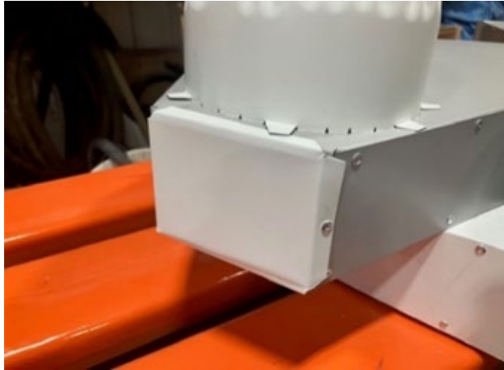
Figure C-18. Plenum End Cap.
