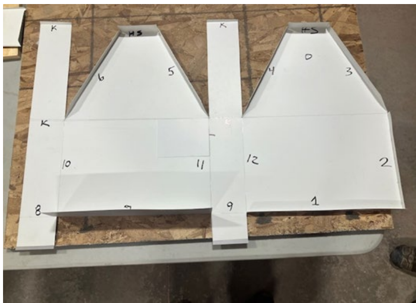
Figure C-8. Plenum Blank with Bends Up.
