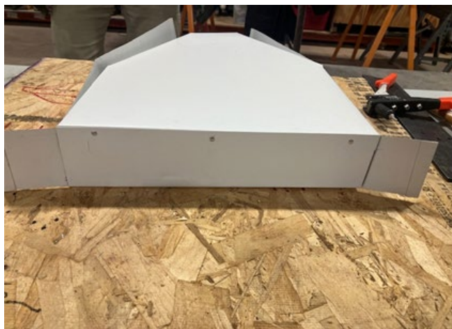
Figure C-12. Plenum with Bottom Secured.
