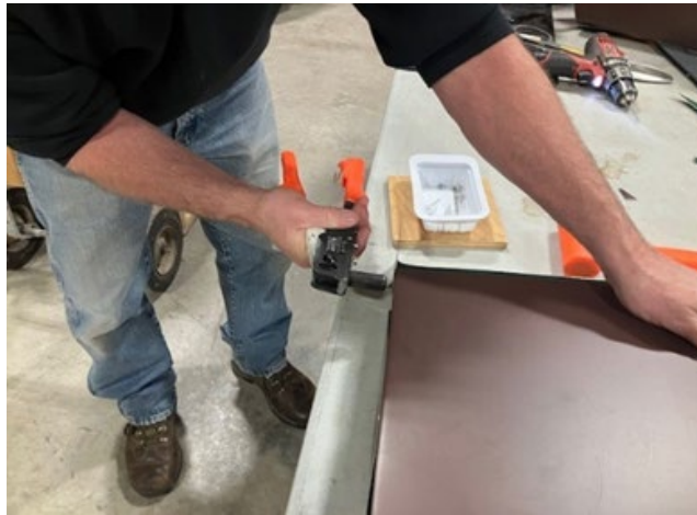
Figure C-13. Secure All Remaining Bent Edges.
