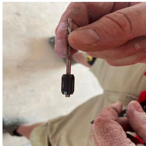
Figure 14-2. Proper Saw Bit Insert Depth.
