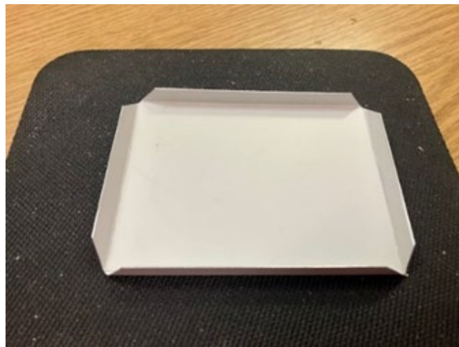
Figure C-15. Plenum End Cap with Notches.
