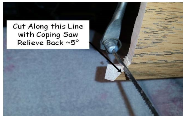
Figure 19-8. Coping Saw Cut.
