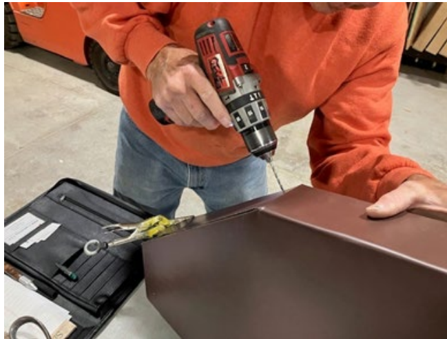
Figure C-11. Drilling Rivet Holes.
