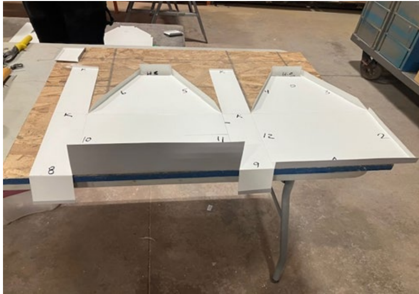
Figure C-9. Plenum Blank with Bends Down.
