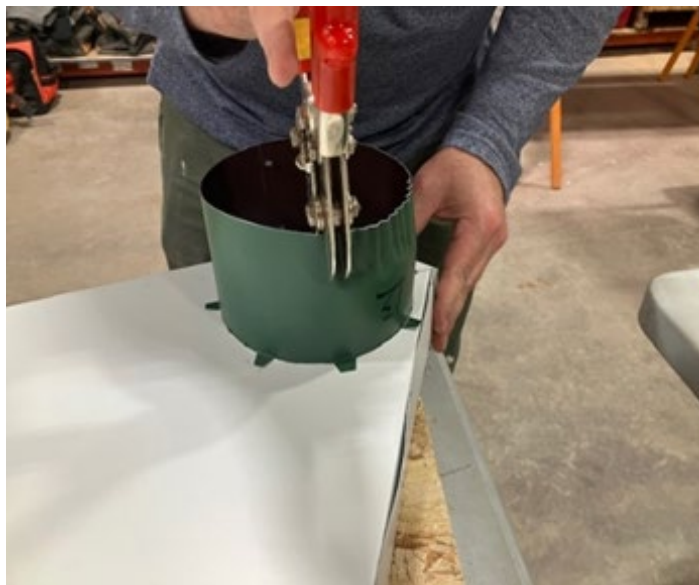
Figure C-17. Crimping Exhaust Pipe.
