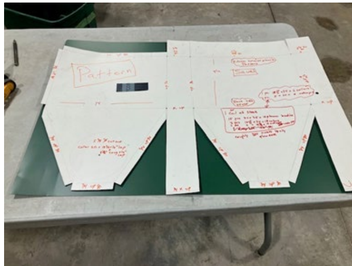
Figure C-1. Pattern on Precut Coil Stock.
