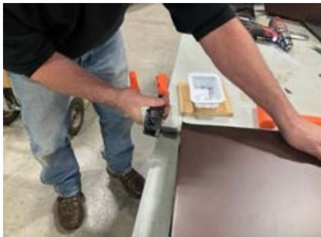
Figure C-13. Secure All Remaining Bent Edges.
