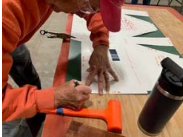
Figure C-4. Highlight Bend Lines.
