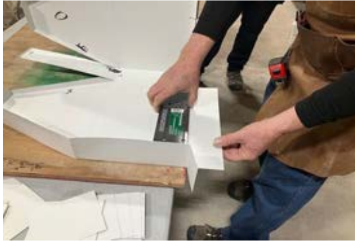
Figure C-10. Bend Plenum Edges to Form a Box.
