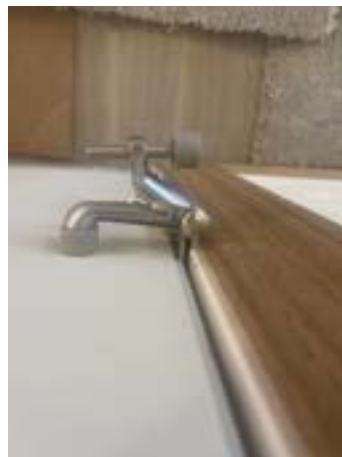
Figure 18-1. Correct Bumper Orientation.
