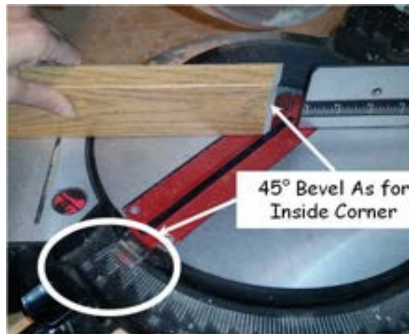
Figure 19-5. Base Trim Bevel Cut.
