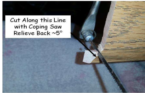
Figure 19-4. Coping Saw Cut.
