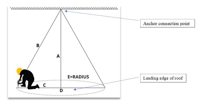
A – is the distance the anchor connection is from the roof edge (leading edge).
